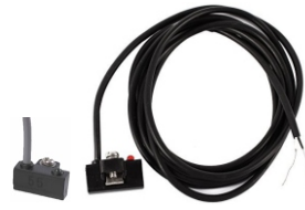
Model - CS1-J Air Cylinder Red LED Light Magnetic Sensor Switch DC/AC 5-240V 100mA 10W
